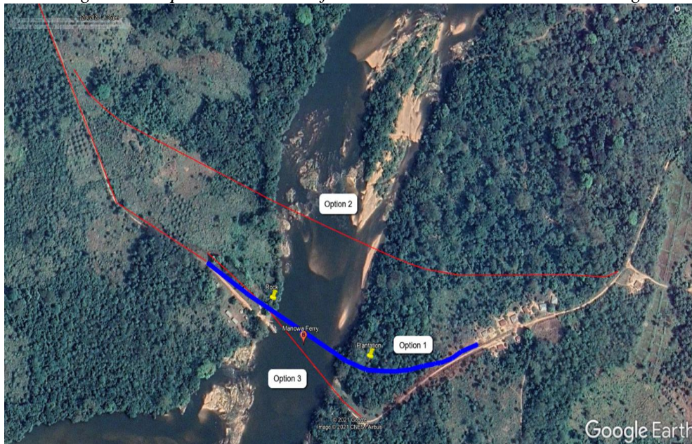
Figure 27: Options considered for the Manowa – Pendembu Crossing
